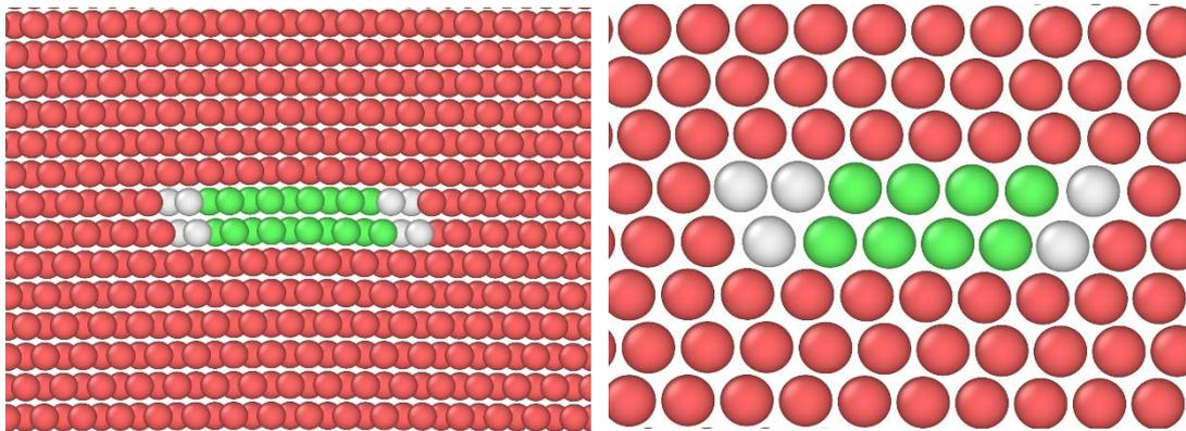
Figure 2: Core structures of the basal  $\langle a \rangle$  dislocation in edge (left) and screw (right) orientations calculated using GPT. The splitting width into partials is consistent with DFT calculations and EAM except in the case of the edge which EAM predicts to have a width twice the DFT value. This shows the value of using quantum mechanics in deriving interatomic potentials.
