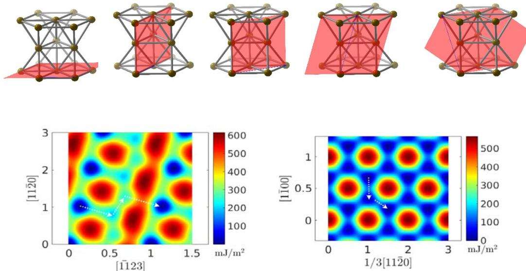
Figure 1: Gamma surfaces on pyramidal I and basal planes in Mg. These show a contour plot of the work needed to slide one half of the crystal over the other. The low contour paths dictate the structure of the dislocations.
