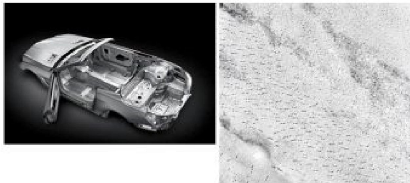
New advanced high strength steels used to reduce the weight of the body in white The transmission electron microscope shows the nanoprecipitates in the steel
